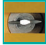
STAINLESS NOZZLE AFTER 50 HOURS
