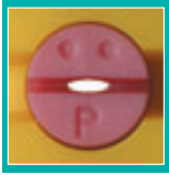
CERAMIC NOZZLE AFTER 50 HOURS
